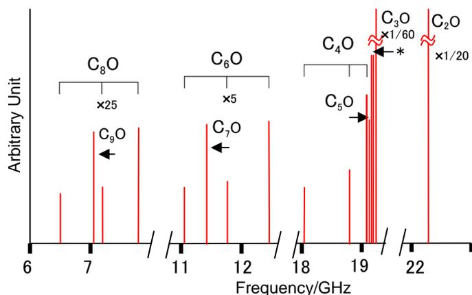
Fig. 1. Rotational spectrum of  $C_nO$  ( $n=2\sim 9$ ) exhibit triplet spectrum for even  $n$  and singlet for odd  $n$ . The vertical scales for  $n = 2, 3, 4$  and  $5, 6$  and  $7$ , and  $8$  and  $9$  are factored by  $1/20, 1/60, 1, 5, 25$ , respectively. The lines marked \* are  $C_3O$  for the  $^{13}C$  species.
