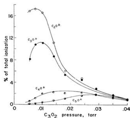
Fig. 3. Pressure dependence of relative abundances of C<sub>m</sub>O<sup>+</sup> ions formed from electron impact in C<sub>3</sub>O<sub>2</sub><sup>3</sup>. Stepwise insertions of a carbon atom lengthened the carbon chains.
