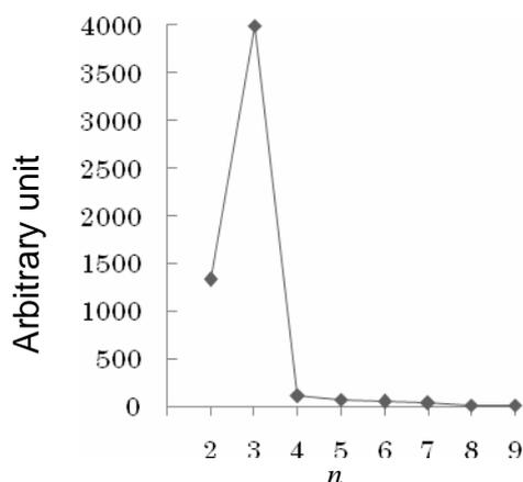
Fig. 2. Relative abundances of C<sub>n</sub>O ( $n=2\sim 9$ ) produced by the discharge of C<sub>3</sub>O<sub>2</sub>.
